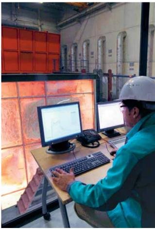
FIRESWISS COOL's performance characteristics are protection against smoke and flame as well as effective protection against the dangerous temperature increase on the side facing away from the flames, so that escape and rescue routes remain accessible even after the fire has been burning for some time.
